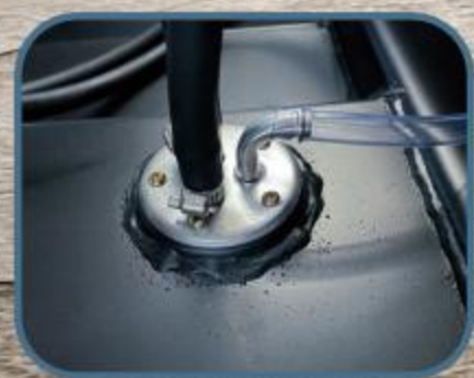
Fuel inlet and return pipe
